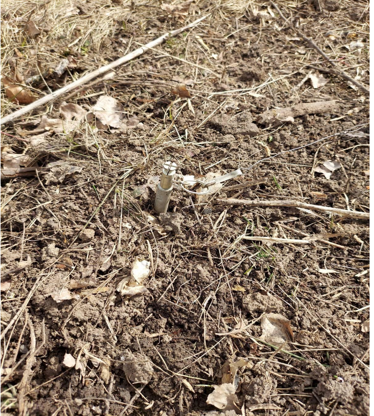
April 2022, City of Trostyanets, Sumy Region Armed OZM-72 Bounding type anti-personnel mine
